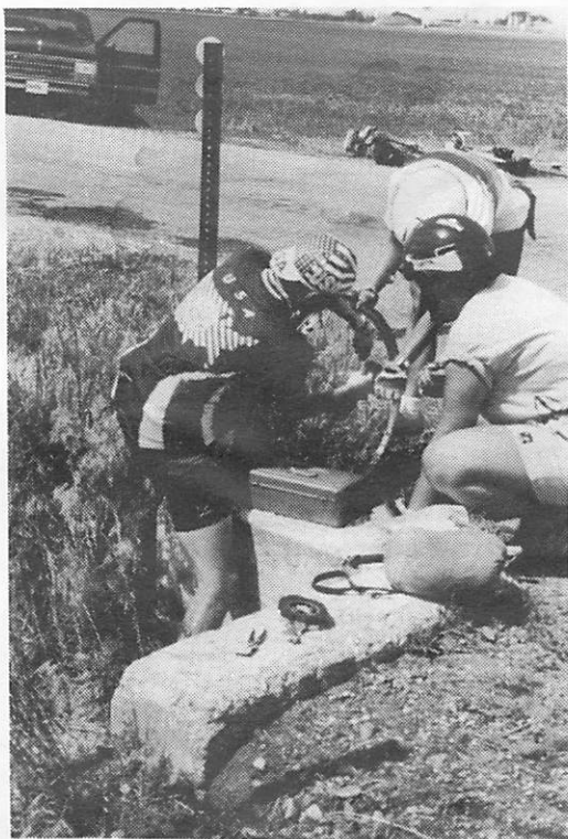
Riders working on tandem wheel trying to remove Phil Wood hub to remove broken spoke behind it.
